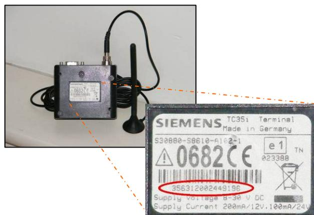
Figure 6.2: Back of the TC35i modem and location of the IMEI
